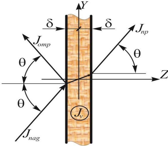
**Fig.4:** The Scheme of Sound Stream Passage through Sheet Material.  $\delta$  – Half Of Sheet Material Thickness,  $\theta$  – The Angle of the Sound Stream Incidence,  $J_{nag}$  – The Energy of the Incident Sound Stream,  $J_{omp}$  – the Energy of the Reflected Sound Stream,  $J_{np}$  – The Energy of the Sound Flow That Passed through the Sheet Material,  $J_v$  – the Energy of the Sound Stream Absorbed by Sheet Material.
