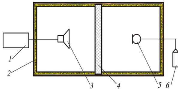
**Fig. 6:** Experimental unit to determine the Sound Insulation of SSLWSP Panels. 1 - the generator of Sound Frequencies; two - muffled chamber; three - sound source; four - Examined Structure; Five - Microphone; Six - Sound Level Meter.
