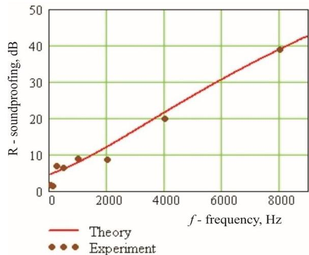
**Fig. 8:** Representation of Theory and Experiment for SSLWSP-3/1 Panel.
