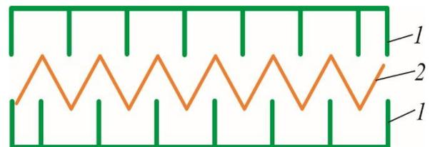
Fig. 2: Main Elements of SSLWSP Panel. 1 – External Element, 2 – Average Layer.
