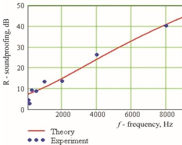
**Fig. 7:** Representation of Theory and Experiment for SSLWSP-2 Panel.
