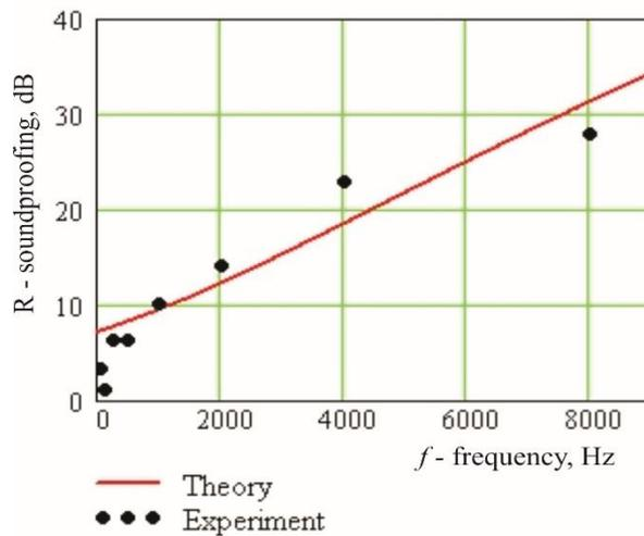
Fig. 9: Representation of Theory and Experiment for SSLWSP-4 Panel.
