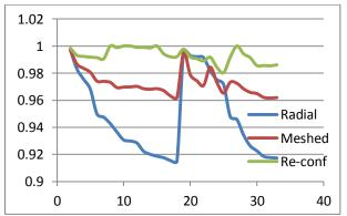
Fig. 8: Comparison between Voltage Profiles of Radial, Weakly Meshed and Reconfiguration Systems.
