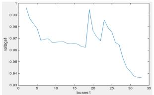
Fig. 4: Voltage Profile of Meshed System when  $B_{33}$ ,  $B_{34}$  and  $B_{35}$  Tie Switches are Closed.
