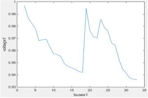
Fig. 2:- Voltage Profile of Meshed System when B<sub>33</sub> Tie Switch is Closed.
