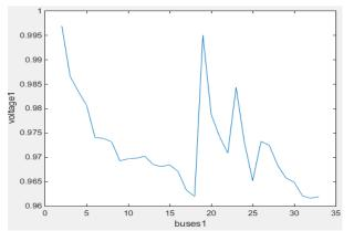
Fig. 6: Voltage Profile of Meshed System when All  $B_{33},\,B_{34},\,B_{35},\,B_{36}$  and  $B_{37}$  Tie Switches Are Closed.
