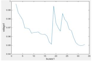
Fig. 5: Voltage Profile of Meshed System when  $B_{33}$ ,  $B_{34}$ ,  $B_{35}$  and  $B_{36}$  Tie Switches Are Closed.
