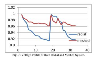
The voltage profile is improved when all the tie switches are closed and the system losses are reduced when compared to system in radial form.
