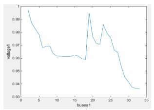
Fig. 3: Voltage Profile of Meshed System when  $B_{33}$  and  $B_{34}$  Tie Switches Are Closed.
