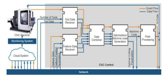
Fig.5: Cloud Architecture of CNC Simulator
