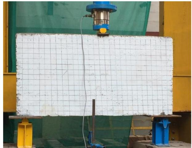
**Fig. 3:** The test set up for deep beams
