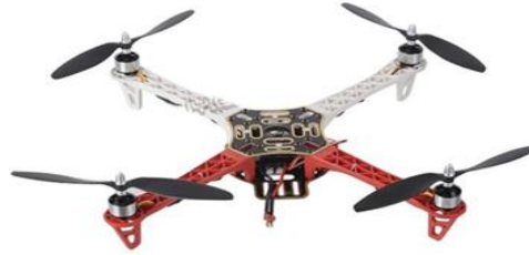
Fig. 1: A quadcopter has four rotors at four corners and a central control unit
