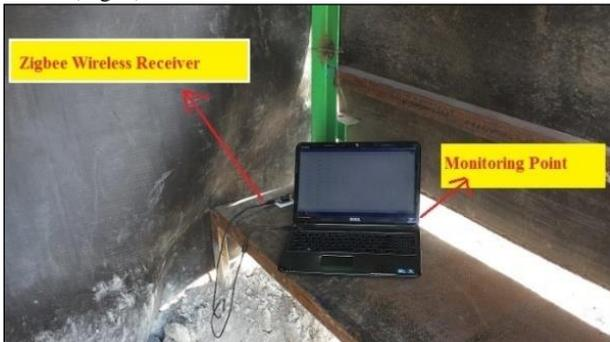
Fig. 4: Remotely monitoring in the field by Zigbee based WDAQ
