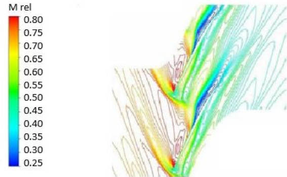
Figure 10: Mach number distribution on stage at Mach 0.8
