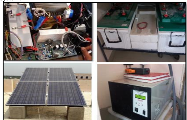
Fig. 8: Hardware implementation of PV system
