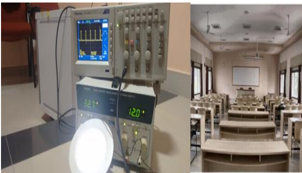
Fig. 10: At 11am: LED is glowing at minimum brightness (duty cycle 10%)
