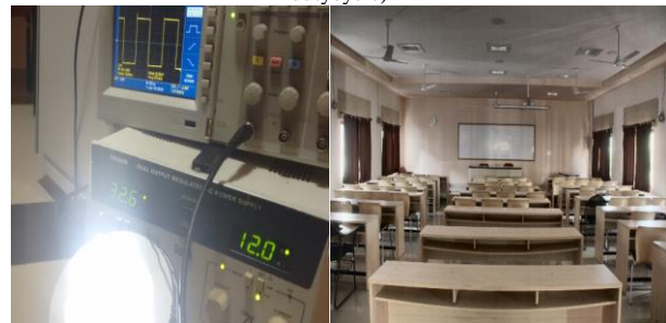
Fig. 12: At 3pm: LED is glowing at medium brightness(50% dutycycle)
