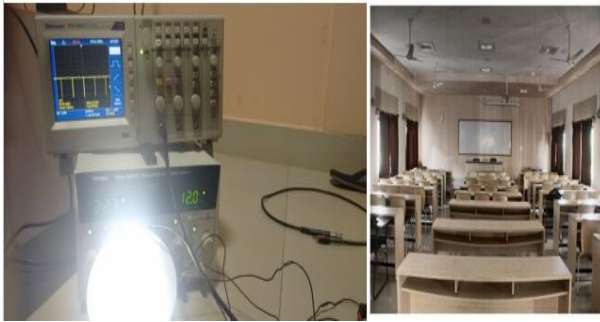
Fig. 9: At 5 pm : blinds closed, LED glowing at its maximum brightness(99%)
