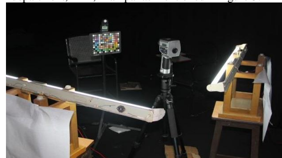
Fig. 3: Experimental setup for the camera calibration
