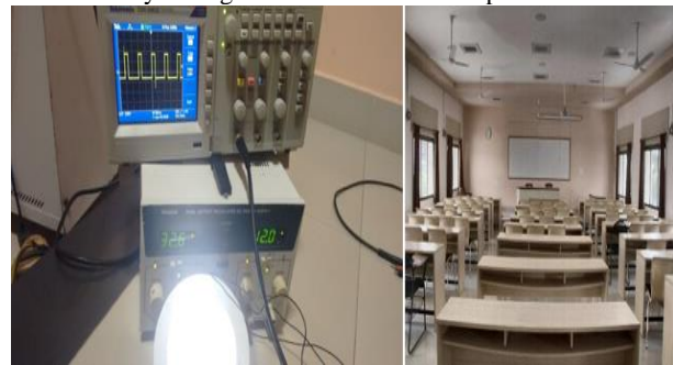
Fig. 11: At 1pm: LED is glowing at medium brightness(25% dutycycle)
