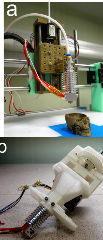
Fig.2: FDM printheads: standard E3D hot end for 1.75 polymer filament (a) and screw extruder for polymer powder (b).
