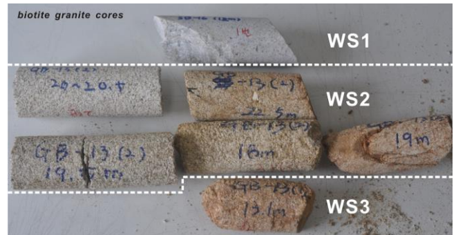
Fig. 1: Photograph of biotite granite cores obtained from the Daejeon area. WS1, WS2, and WS3 represent weakly, moderately, and strongly weathered granites, respectively. Samples 1, 2, and 3 were analyzed in this study.
