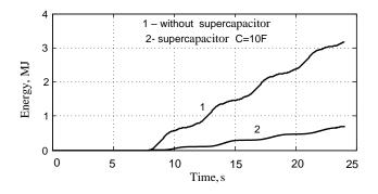
Fig. 8: Diagrams of the consumption of electric energy in the system without a supercapacitor (line 1) and with a supercapacitor (line 2)
