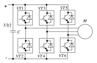
Fig. 4: The converter circuit for controlling induction motor
