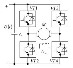
Fig. 3: The converter circuit for controlling DC motor
