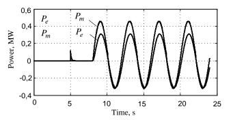
Fig. 5: Diagrams of the electrical  $P_e$  and mechanical  $P_m$  power of the motor
