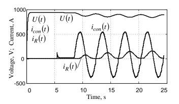
**Fig. 6:** Diagrams of the processes in the DC link: U(t)- voltage at the supercapacitor;  $i_R(t)$  - current at the output of the rectifier;  $i_{con}(t)$  - current at the input of the inverter
