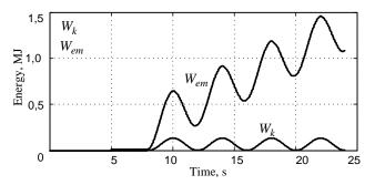
Fig. 7: Diagrams of the energy processes:  $W_k$  - kinetic energy of the oscillating masses;  $W_{em}$  - electric energy consumed by the engine
