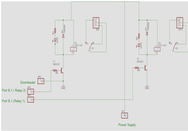
Fig.4: Relay Circuit
