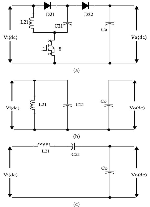
Fig. 2: (a) Overall circuit of the SLC, (b) SLC during switch ON, and (c) SLC during switch OFF
