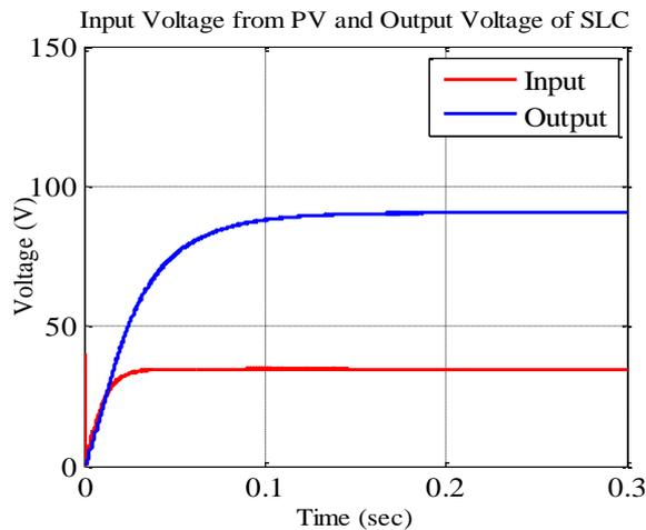
Fig. 8: Input Voltage from PV and Output Voltage of SLC
