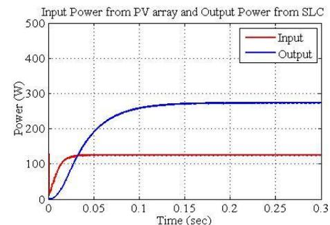
Fig. 7: Input Power from PV array and output Power from SLC
