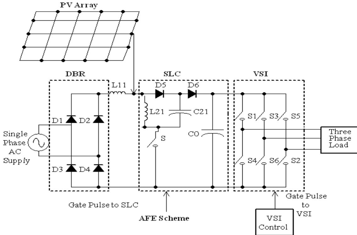
Fig. 1: Schematic of the proposed system
