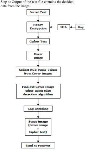
Fig. 2: Block diagram for encoding process
