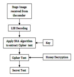
Fig.3: Block diagram for decoding process
