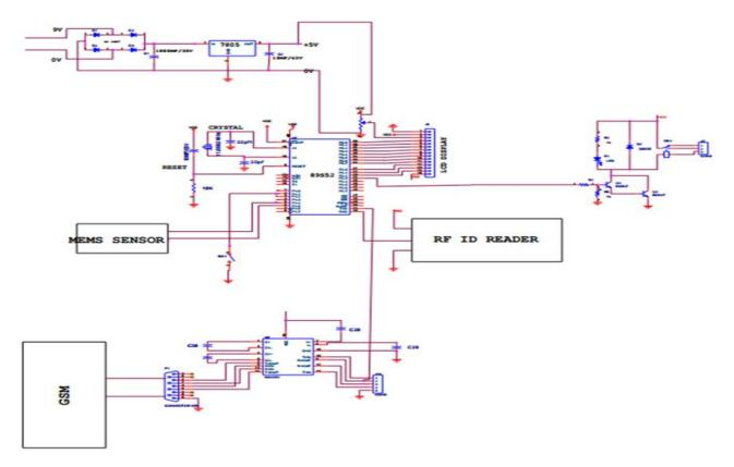
Fig. (c): Circuit diagram of a proposed system
