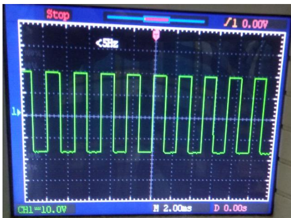
Fig. 26: Primary voltage of Transformer
