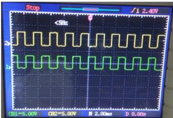
Fig. 25: Switching pulses for M1 & M3
