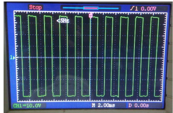
Fig. 27: Secondary voltage of Transformer
