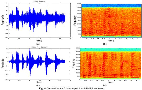
(a) Noisy Speech, (b) Spectrogram of (a), (c) Noise Free Speech, (d) Spectrogram of (c)
