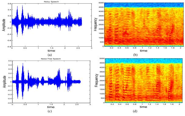
**Fig. 3:** Obtained results for clean speech with Babble Noise, (a) Noisy Speech, (b) Spectrogram of (a), (c) Noise Free Speech, (d) Spectrogram of (c)
