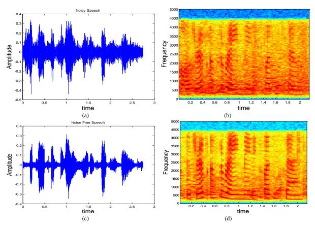
**Fig. 5:** Obtained results for clean speech with Restaurant Noise, (a) Noisy Speech, (b) Spectrogram of (a), (c) Noise Free Speech, (d) Spectrogram of (c)
