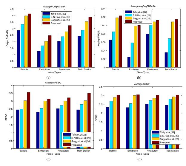
**Fig. 7:** Performance metrics evaluation and comparison, Average value of (a) Output SNR, (b) AvgSegSNR, (c) PESQ and (d) COMP for different noise types
