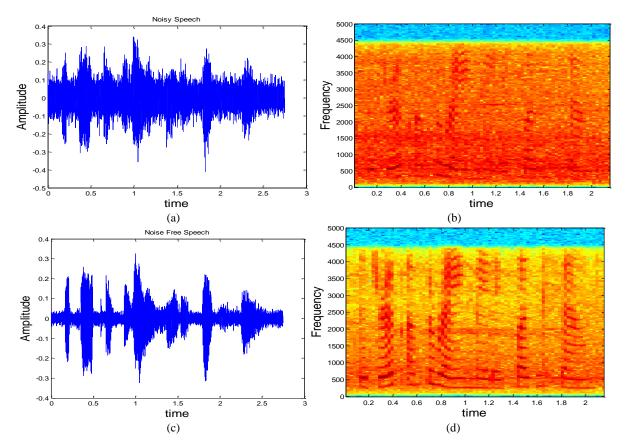
**Fig. 6:** Obtained results for clean speech with Train Station Noise, (a) Noisy Speech, (b) Spectrogram of (a), (c) Noise Free Speech, (d) Spectrogram of (c)
