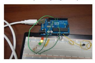
Fig. 5: Temperature Sensor
