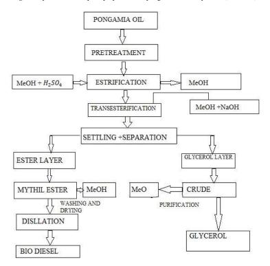
Fig. 2: Flow chart of esterification
