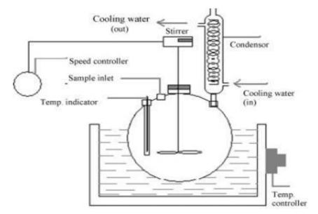
Fig. 1: Experimental setup for preparation of pongamia oil methyl ester (Biodiesel)
