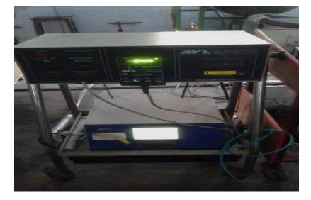
Fig. 6: Emission Sensing Unit
