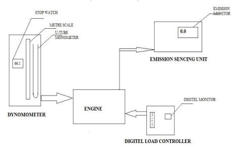
Fig. 7: Block Diagram of Experimental Engine setup
