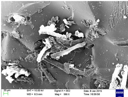
**Fig. 4:** SEM micrograph of tensile fracture surface of sample 4. Micrograph of sample 4 shown in figure 4. The failure of sample 4 is mainly due to the presence of voids and improper mixing of fiber and fly ash.
