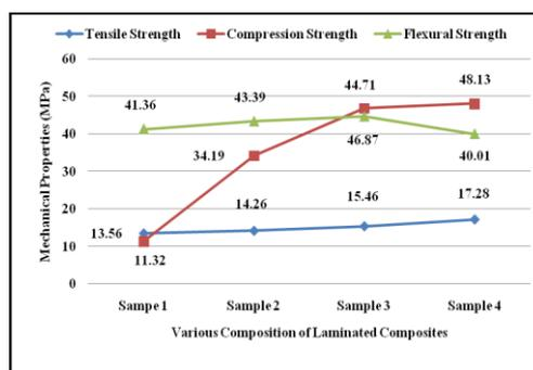
**Graph 1:** Mechanical properties of various laminated samples
