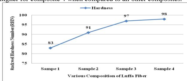
**Graph 2:** Rockwell hardness values of various laminated samples
