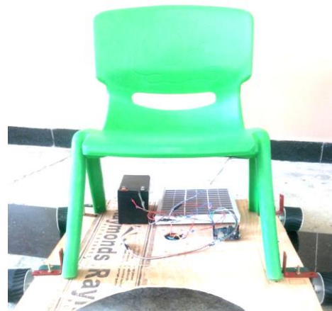
Fig. 5: Wheel chair board top view connected with all components Multipurpose multi module wheel chair
