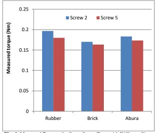
Fig. 4: Measured Torques for Same Screw Type with Different Sizes.
