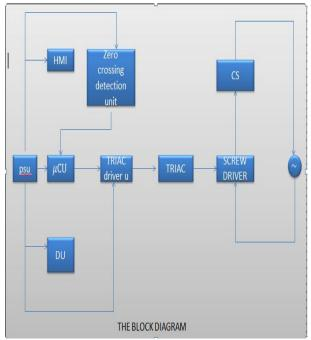
Fig. 1: The Block Diagram for Controller Unit.
