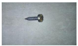
Fig. 9: Phillips Pan Head Brass Coated Screw.
