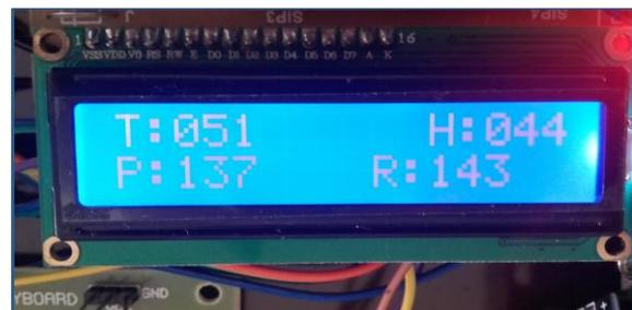
Fig. 6: Sensor values displayed on LCD
