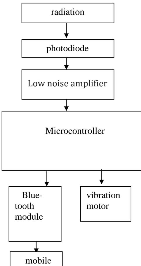
Fig.1. Block diagram of radiation detector
