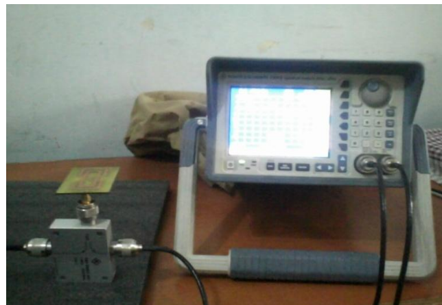
Fig.9: Setup for measurement of antenna parameters.
