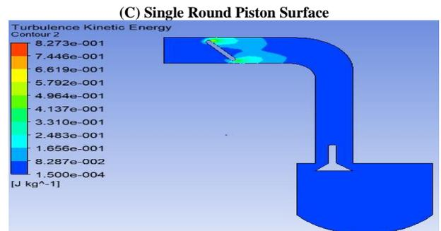
Fig. 6: The Turbulence Kinetic Energy with Different Piston Shapes at 45 Degrees.
