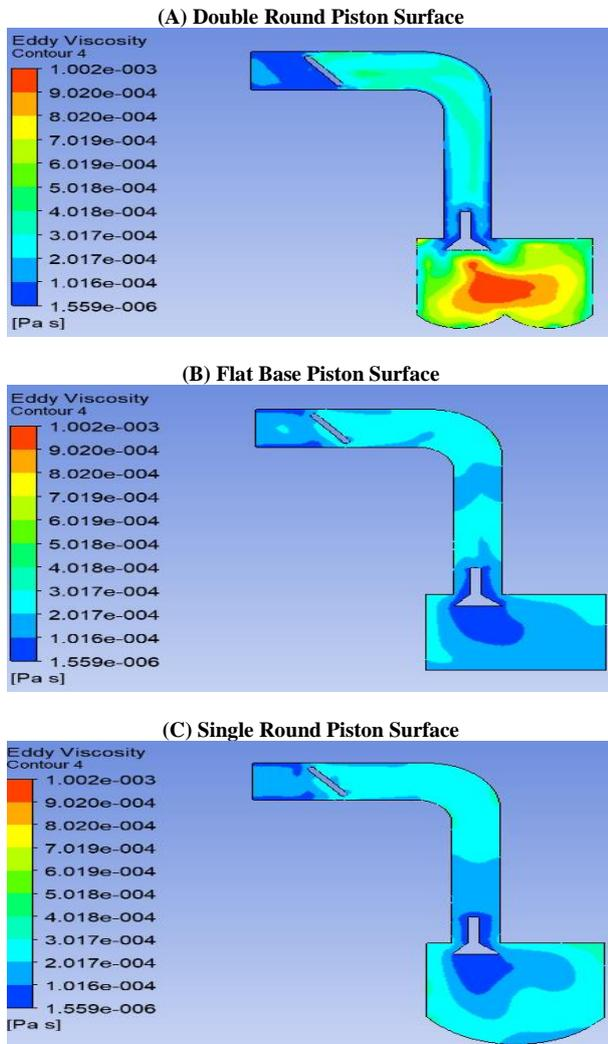
Fig. 7: The Eddy Viscosity with Different Piston Shapes at 45 Degrees.
