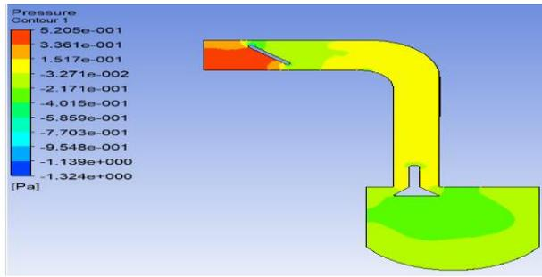
Fig. 2: The Pressure with Different Piston Shapes at 30 Degrees.
