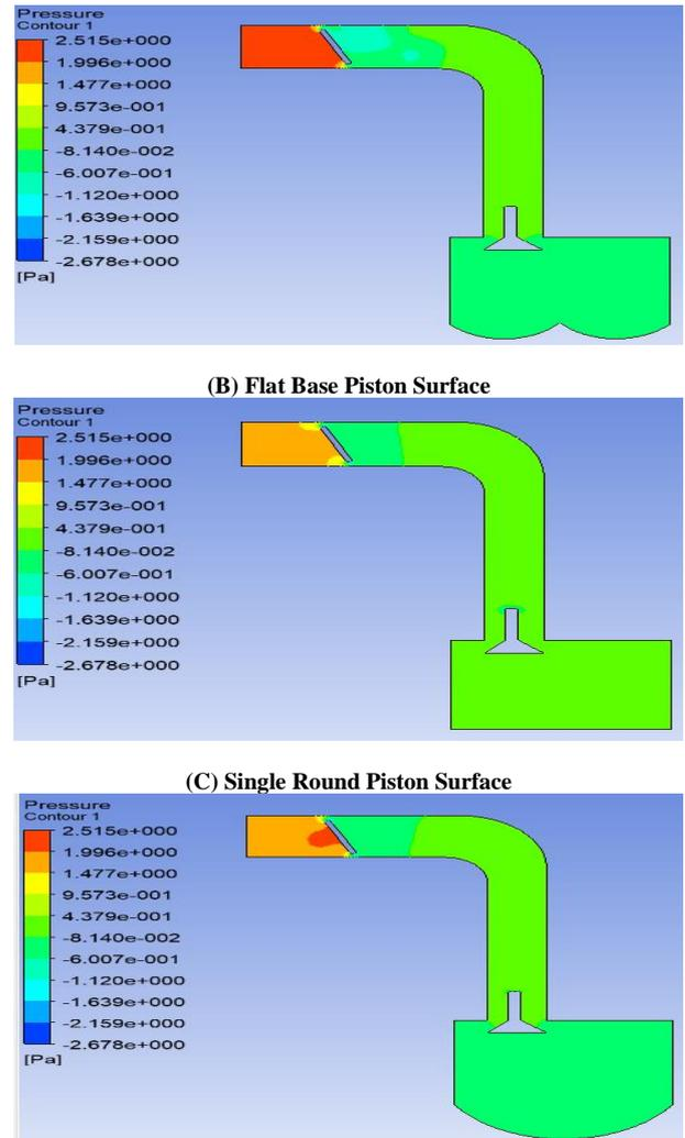
Fig. 8: The Pressure with Different Piston Shapes at 60-Degree Angle.
