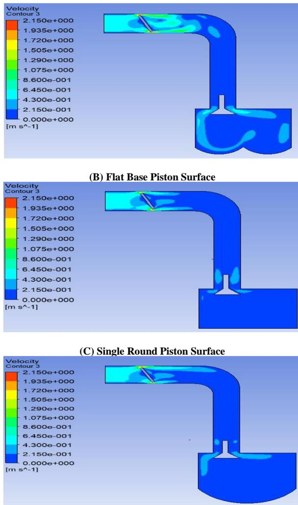
Fig. 9: The Velocity with Different Piston Shapes at 60-Degree.
