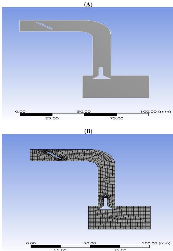
Fig. 1: The Basic Model of Simulation with 30° Angle.
