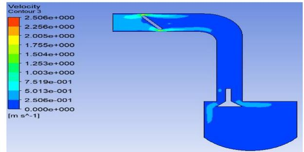
Fig. 5: The Velocity with Different Piston Shapes at 45 Degrees.
