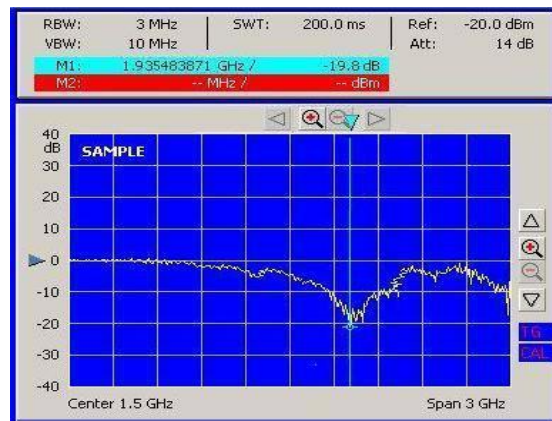
Fig. 10 Measured resonant frequency of liquid monopole antenna at specific salinity (3 M)
