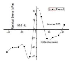
Fig. 8: Residual Stress in Pass-1.
