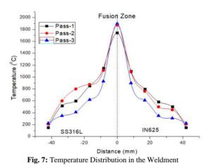
It has been observed that the SS metal has high thermal conductivity as compared to Inconel, which tends the SS to contract more during solidification which results in generation or development of compressive stress. Whereas, in Inconel side was higher resistant material and low thermal conduction value, resulting production less in stresses as compared to SS side.
