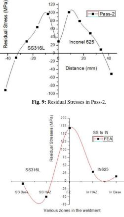
Fig. 10: Residual Stresses in Pass-3.
