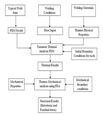
Fig. 1: Flowchart of the Sequentially Coupled Thermo-Mechanical Analysis Procedure.
