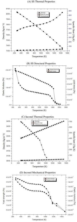
Fig. 3: Thermal and Mechanical Properties of SS and Inconel 625 Base Materials.
