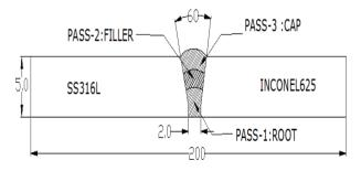
Fig. 2: Multipass-Welding Process.
