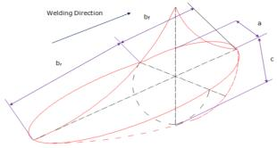
Fig. 4: Double Ellipsoidal Heat Flux.
