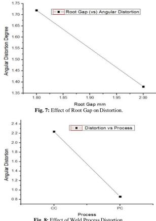
Fig. 8: Effect of Weld Process Distortion.
