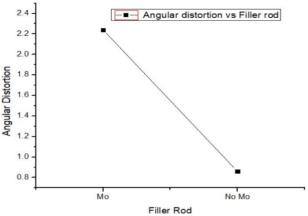
Fig. 9: Effect of Filler Wire on Distortion.
