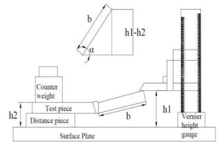
Fig. 4: Schematic Representation of Measurement of Distortion Using Vernier Height Gauge.
