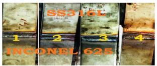
Fig. 2: GTA Welded Samples.
