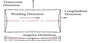
Fig. 3: Distortion Caused by Welding.
