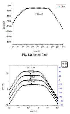
Fig. 13: Simulation result of programmable gain amplifier
