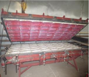
Fig. 10: Clay Plate Mould.
