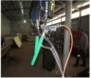
Fig. 11: Equipment for the Manufacture of Rigid Polyurethane Foam.
