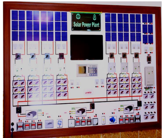
Fig. 14: Practical board of solar power plant.
