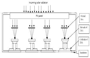
Fig. 6: PV-TE Indirect Coupled PV-TE System.
