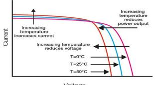
Voltage Fig. 3: Characteristics Curve for PV Cell [3].
