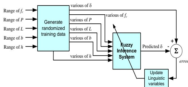
Fig. 7: Training process for modeling of deflection prediction using FIS
