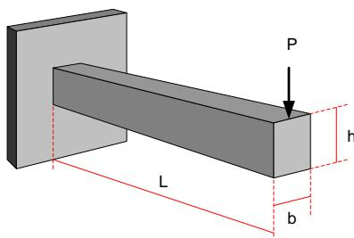
Fig. 1: Cantilever Beam.
