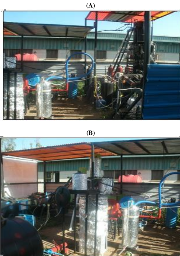
Fig. 1: (A, B) the Text System of Adsorption Materials and Tanks of Al-Masaya Industrial Water.
