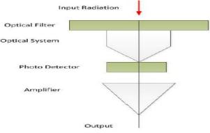
Fig. 4: Flow Diagram of VLC Communication.
