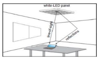
Fig. 5: Implementation of Visible Light Communication System.
