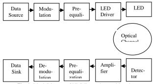
Fig.1: Block Diagram of VLC Transmitter and Receiver.
