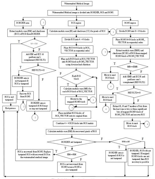
Fig. 9: ROI Authentication and Recovery Process.
