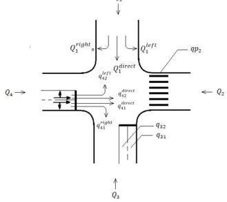
Fig. 3: Notations of the movement of traffic and pedestrian flows through the intersection
