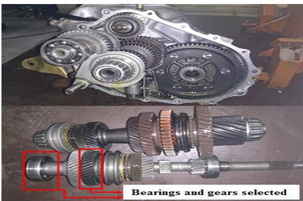
Fig. 3: Interior View of the Gearbox to Display the Selected Bearings and Gear for Testing.
