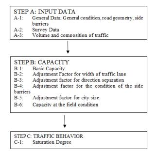
Fig 2:. Flow Chart of the calculation analysis of urban road segment performance
