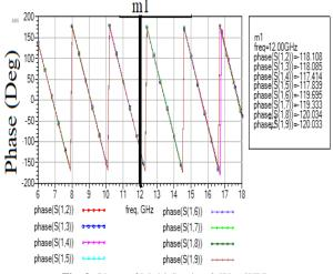
Fig. 9: Phase of Multi-Section 8-Way WPD.
