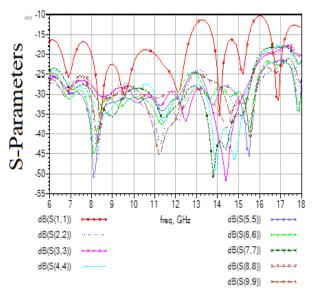
Fig. 6: Return Loss of Multi-Section 8-Way WPD.
