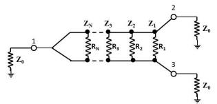
Fig. 2: General Circuit for Multiple-Section Three Ports WPD [4].
