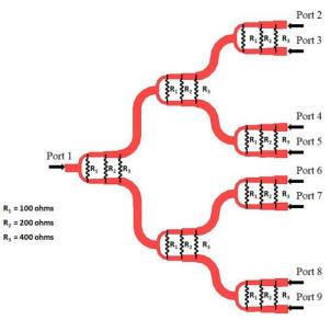
Fig. 5: Layout Diagram of Multi-Section 8-Way WPD.
