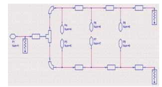
Fig. 4: Schematic Diagram of Single Multi-Section 2-Way WPD.
