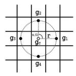
**Fig. 5:** Center pixel  $g_c$  and its 4 circular neighbours  $\{g_i\}_{i=0}^{3}$  with radius r for the LBP operator.
