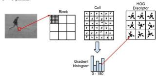
Fig. 4: Block diagram of HOG method.
