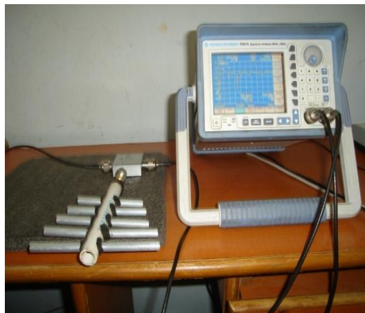
Figure2. Measurement set up to measure return loss of designed yagi-uda antenna
