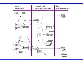
Fig 2. GSM System architecture
