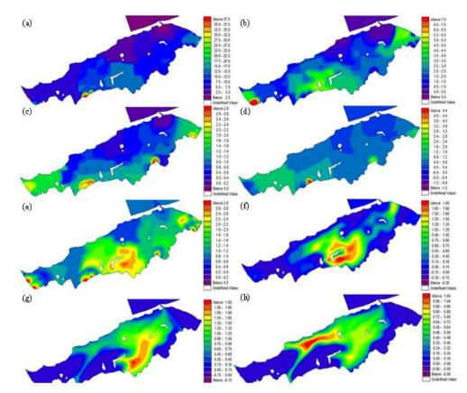
Fig. 6: Simulation of Water Quality Parameters by MIKE21 Software: Calibration Procedure for (A) BOD, (B) NH<sub>3</sub>-N, (C) NO<sub>3</sub>-N, and (D) PO<sub>4</sub>-P, As Well as, Enhancement Scenario for (E) BOD, (F) NH<sub>3</sub>-N, (G) NO<sub>3</sub>-N, and (H) PO<sub>4</sub>-P.
