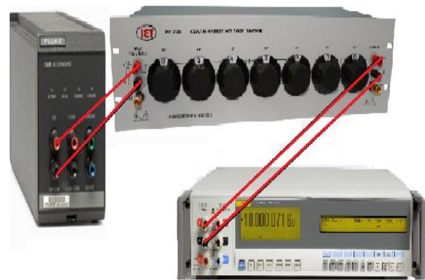
Fig. 1: Calibration Setup of ESI RV-722 Voltage Divider.
