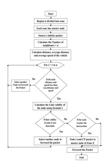
Fig. 1: Flow Chart of Geographical Zone Based Routing for Sparse Networks.
