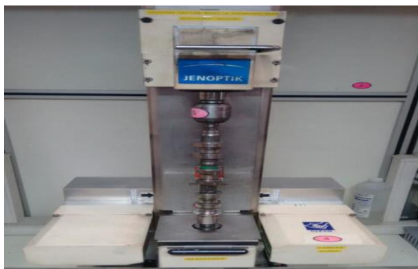
Fig 2: Surface Roughness Measurement Setup.
