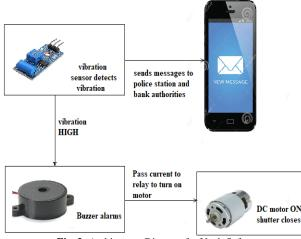
Fig. 3: Architecture Diagram for Vault Safety
