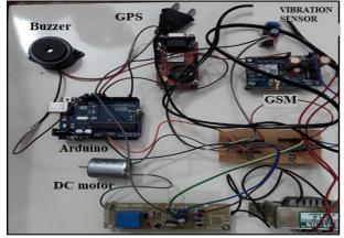
Fig. 10: Result of Physical Attack Detection Module.
