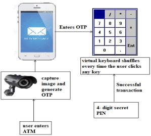
Fig. 2: Architecture Diagram for PIN Safety
