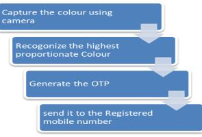
Fig. 4: User Authentication Module Flow Diagram.
